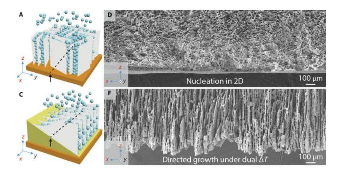
SEM images of xz cross-sections perpendicular to the cold finger show that in conventional freeze-casting (A&D), nucleation produces a disordered layer of ceramic particles. Under bidirectional freeze-casting (C&F), with dual temperature gradients, ice crystals grow both vertically and horizontally into a well-aligned lamellar structure. Credit: Berkeley Lab
