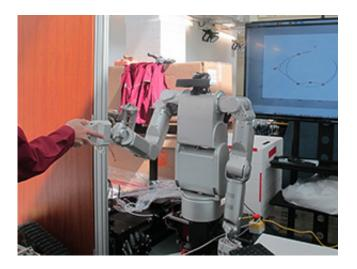
A role adaptation control scheme allows the leader or follower role of a robot to be adjusted continuously based on the sensed intention of a human collaborator. Credit: A\*STAR Institute for Infocomm Research
