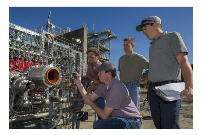
Engineers prepare a 3-D printed breadboard engine made up of 75 percent of the parts needed to build a rocket engine for a test at NASA's Marshall Space Flight Center in Huntsville, Alabama. Credit: NASA/MSFC/Emmett Given
