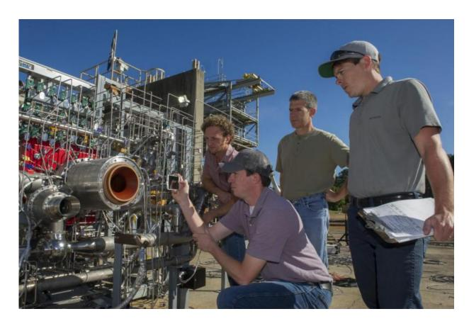
Engineers prepare a 3-D printed breadboard engine made up of 75 percent of the parts needed to build a rocket engine for a test at NASA's Marshall Space Flight Center in Huntsville, Alabama. Credit: NASA/MSFC/Emmett Given
