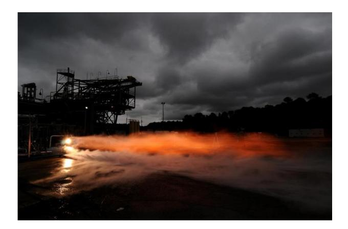
During a series of test firings at NASA's Marshall Space Flight Center in Huntsville, Alabama, 3-D printed rocket engine parts worked together successful under the same conditions experience inside rocket engines used in space. The turbopump was tested at full power, pumping 1,200 gallons of liquid hydrogen per minute and the injector produced 20,0000 pounds of thrust. Credit: NASA/MSFC/David Olive
