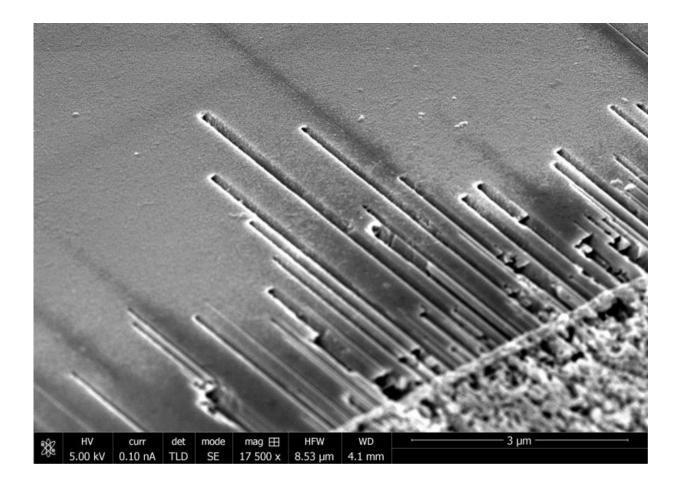
Electron micrograph of surface-directed nanochannels formed on the surface of the semiconductor indium phosphide. Nanochannels are formed using a goldcatalyzed vapor-liquid-solid etch process and their locations are defined by the deposited gold pattern. Credit: NIST/Nikoobakht
