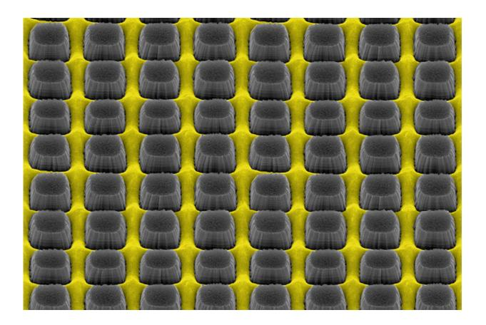
An array of nanopillars etched by thin layer of grate-patterned metal creates a nonreflective surface that could improve electronic device performance. Credit: Daniel Wasserman
