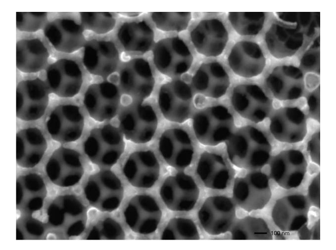
An electronmicroscopical image of the germanium-structure after removal of the polymer templates. The material forms an inverse opal-structure, which can be filled with suitable polymers to create hybrid solar cells. Credit: Katia Rodewald / TUM
