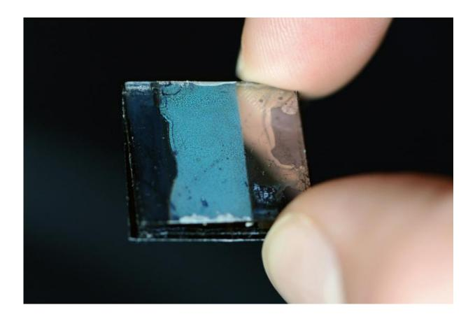
Filled with suitable organic polymers the highly porous germanium nanofilm becomes a hybrid solar cell. Because the germanium nanostructure forms an inverse opal-structure, the material shimmers like opal. Credit: Andreas Battenberg / TUM
