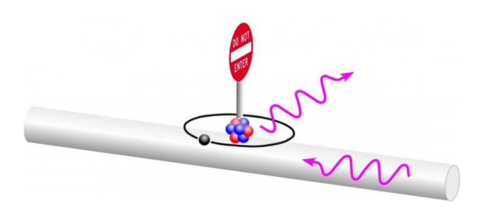
An optical device at nanoscale which allows light to pass in only one direction has been developed at TU Wien (Vienna). It consists of alkali atoms which are coupled to ultrathin glass fibres.
