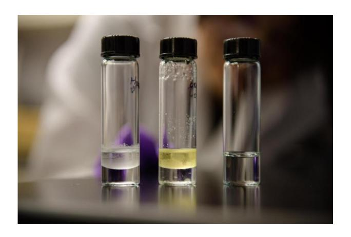
After shaking, the oil and water in the vial separate, trapping unwanted nanomaterials in the bottom of the oil layer. Credit: Michigan Tech, Sarah Bird
