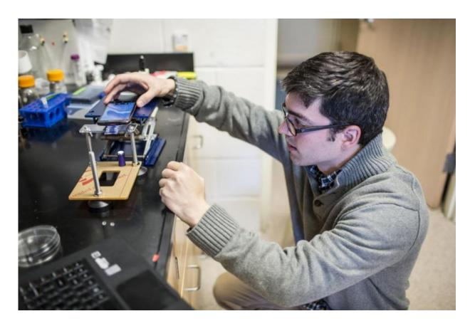
Emory post-doctoral fellow Kevin Yehl sets up a smart-phone microscope to get a readout for the particle motion of the rolling DNA motor. This simple, low-tech method could come in handy for doing disease diagnostics in the field, for instance, detecting a single mutation in a DNA strand. Credit: Bryan Meltz, Emory Photo/Video
