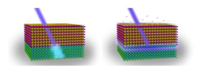
In the presence of a water molecule on its surface, lanthanum aluminate film on a strontium titanate crystal emits ultraviolet light from its interior. (Illustration not to scale). Credit: Drexel University
