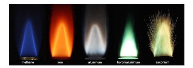
Stabilized flames of different metal powders burn with air, compared to a methane-air flame. Credit: Alternative Fuels Laboratory/McGill University
