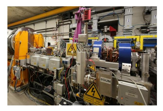
The 'gun' releases the electrons and accelerates them shaped in bunches. Credit: Dirk Nölle, DESY
