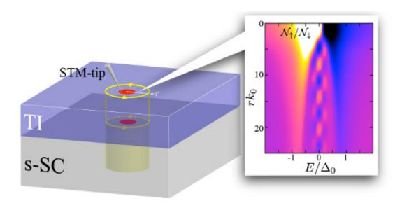
Schematic of Majorana particles localized inside the core of quantum vortex of a topological superconductor and the distribution of density of states of superconducting quasiparticle excitations based on the theoretical calculations.
