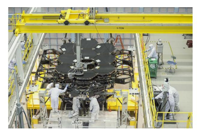
Engineers worked tirelessly to install the ninth primary flight mirror onto the telescope structure. Credit: NASA's Goddard Space Flight Center/Chris Gunn
