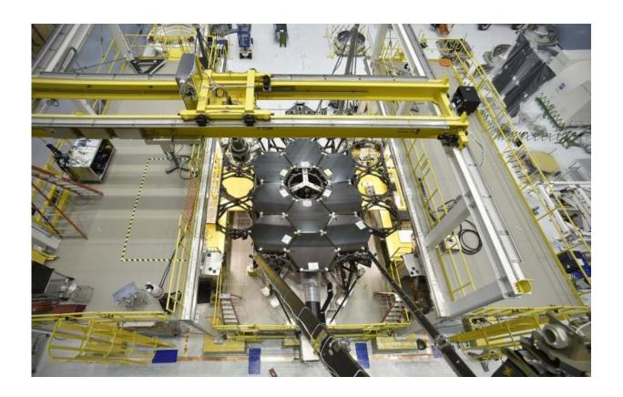
This rare overhead shot of the James Webb Space Telescope shows the nine primary flight mirrors installed on the telescope structure in a clean room at NASA's Goddard Space Flight Center in Greenbelt, Maryland. Credit: NASA's Goddard Space Flight Center/Chris Gunn
