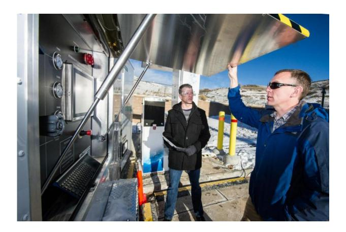
Sandia National Laboratories mechanical engineer Terry Johnson, left, the project leader for the Hydrogen Station Equipment Performance (HyStEP) device, and National Renewable Energy Laboratory researcher Chris Ainscough prepare HyStEP for testing at NREL's Energy Systems Integration Lab. HyStEP will accelerate hydrogen refueling station commissioning. Credit: Dennis Schroeder/NREL
