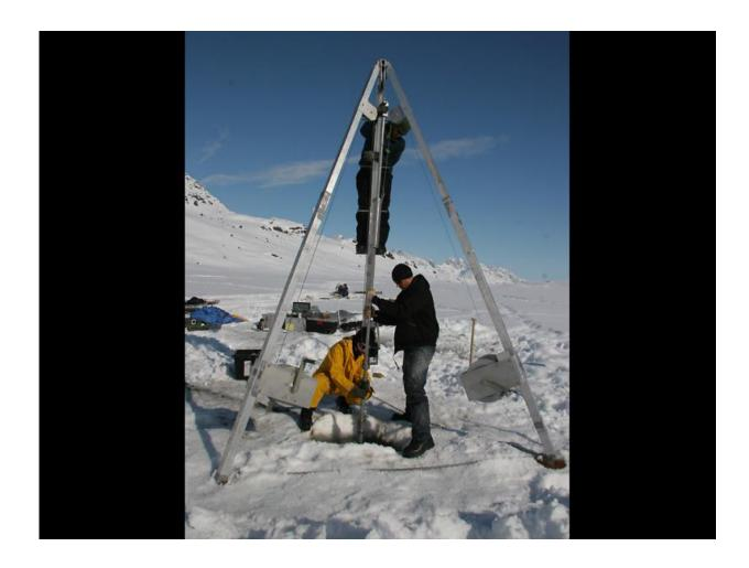
Once the tube is driven into the sediment, special equipment is used to raise the core through 70 meters of water. Credit: William D'Andrea
