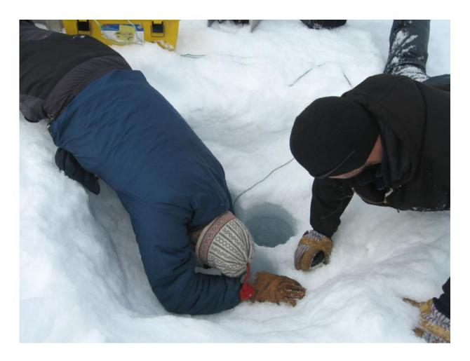
Extracting the sediment core starts with clearing out a hole through the lake's 3-foot-thick ice. Credit: William D'Andrea
