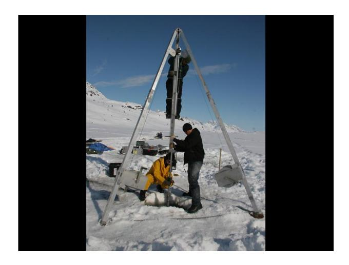
Once the tube is driven into the sediment, special equipment is used to raise the core through 70 meters of water. Credit: William D'Andrea
