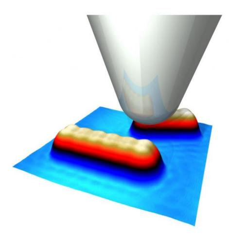
Schematic of the tip of a scanning tunneling microscope on a graphene nanoribbon.
