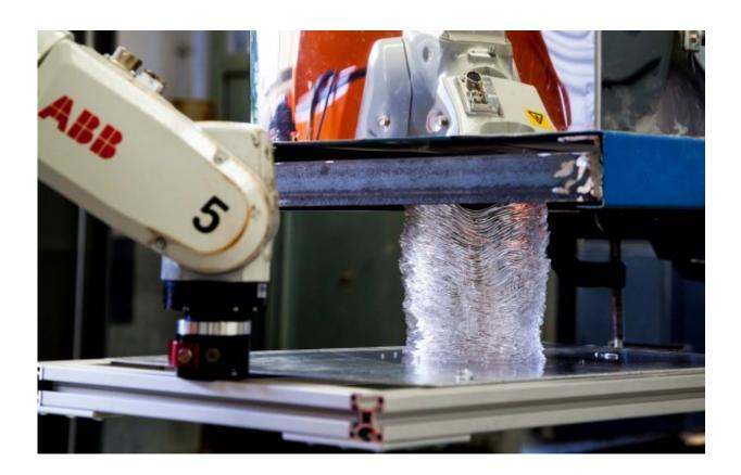
Glass structure created using robot-based 3-D glass printing.
