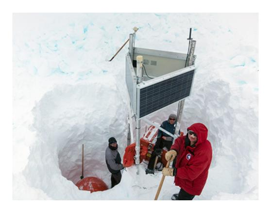
A team maintains a seismic station on Thwaites Glacier, an area of heavy snowfall. The seismometer is in the orange dome in the lowest part of the three-step snow pit. Credit: Mike Roberts
