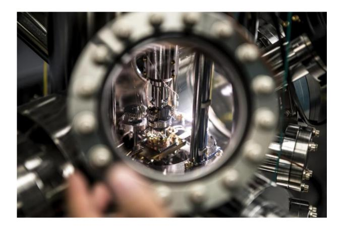
The view inside the Ultra High Vacuum Scanning Thermal Microscope, which was used to measure temperature fluxes at the nanoscale. Credit: Joseph Xu
