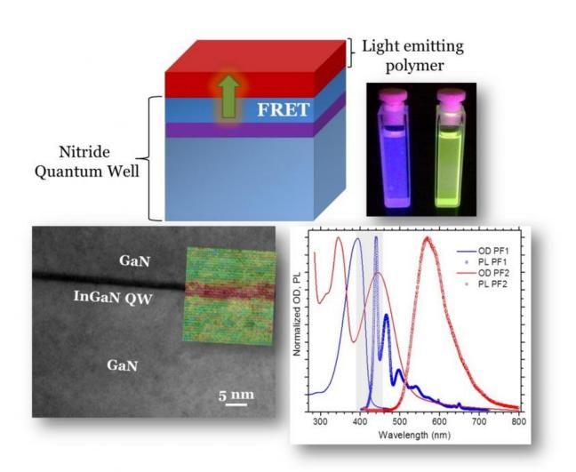
(Top left) Schematic of Förster Resonant Energy Transfer from a near-surface nitride quantum well to a polymer overlayer. (Top right) Fluorescence from solutions containing light emitting polymer materials. (Bottom left) High resolution transmission electron microscope image from an InGaN/GaN
