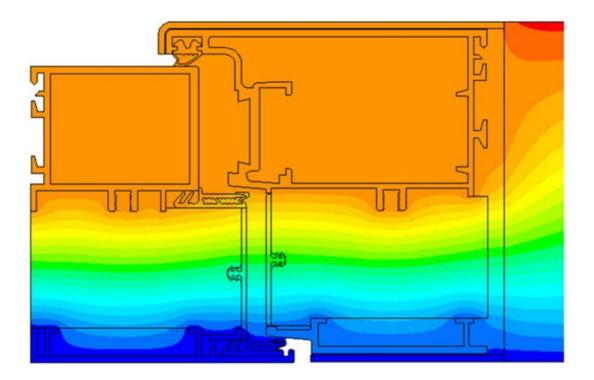
Cross-section of burglary-resistent external doors: Using scientific simulation methods, Fraunhofer researchers have identified the exact points where heat escapes through the aluminum frame (dark color). Credit: Fraunhofer ITWM
