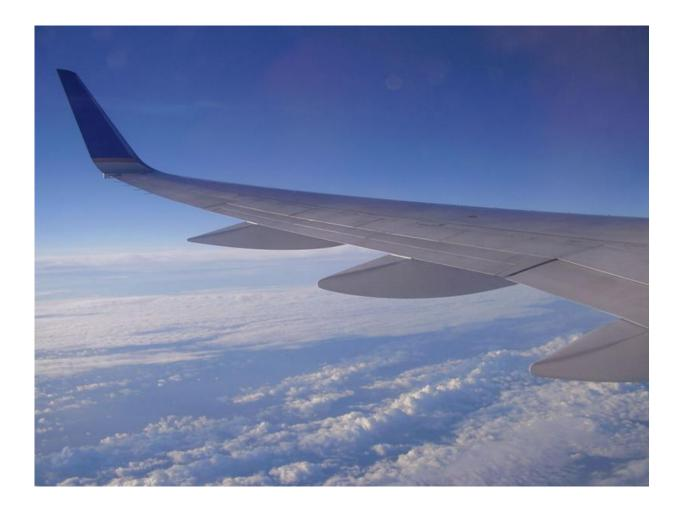
A winglet on the wing tip, designed to reduce drag. Credit: Hecki
