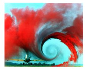
Experiments with smoke reveal strength and size of wingtip vortices. Credit: NASA
