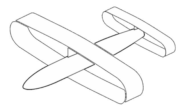
A box wing design, where the upper and lower wing surfaces 'wrap around'. Credit: Steelpillow, CC BY-SA
