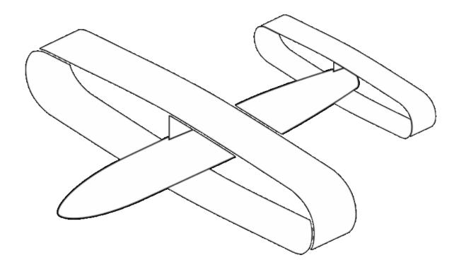
A box wing design, where the upper and lower wing surfaces 'wrap around'. Credit: Steelpillow, CC BY-SA
