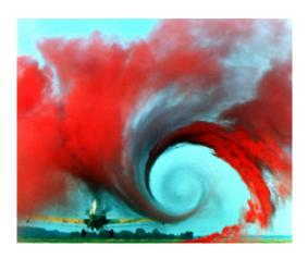
Experiments with smoke reveal strength and size of wingtip vortices. Credit: NASA
