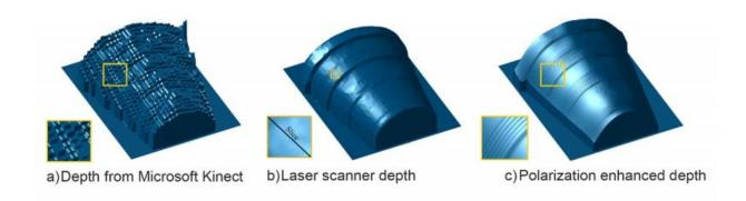
By combining the information from the Kinect depth frame in (a) with polarized photographs, MIT researchers reconstructed the 3-D surface shown in (c). Polarization cues can allow coarse depth sensors like Kinect to achieve laser scan quality (b).
