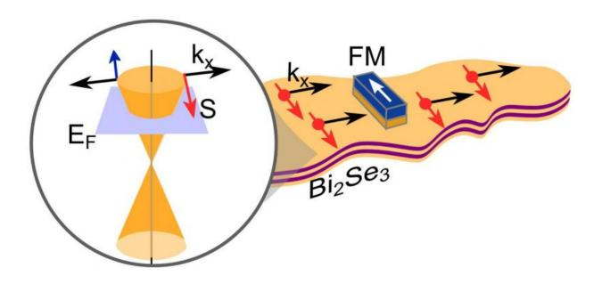
Schematics of the spin current on a topological insulator surface, with the spin direction (S) perpendicular to the current direction (kx). The zoom in schematic shows the electronic band structure on the surface of the topological insulator. The spin polarization on topological insulator surface is electrically probed by a ferromagnetic tunnel contact (FM). Credit: André Dankert
