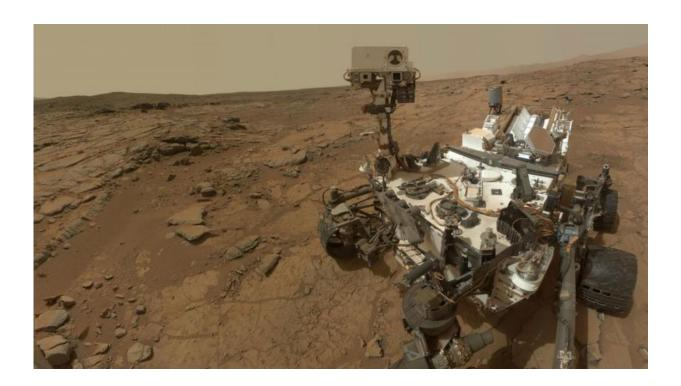
This self-portrait of NASA's Mars rover Curiosity combines dozens of exposures taken by the rover's Mars Hand Lens Imager (MAHLI) during the 177th Martian day, or sol, of Curiosity's work on Mars (Feb. 3, 2013), plus three exposures taken during Sol 270 (May 10, 2013) to update the appearance of part of the ground beside the rover. Credit: NASA/JPL-Caltech/MSSS
