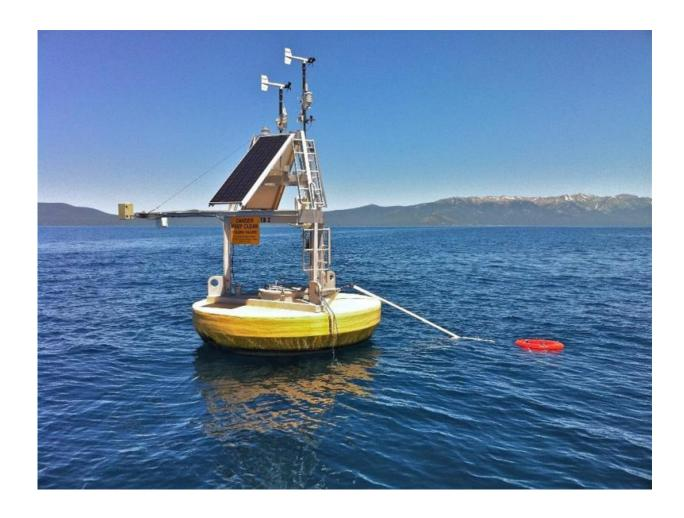
A combination of satellite data and ground measurements, such as from instrumented buoys like this one in Lake Tahoe on the California/Nevada border, were used to provide a comprehensive view of changing lake temperatures worldwide. The buoy measures the water temperature from above
