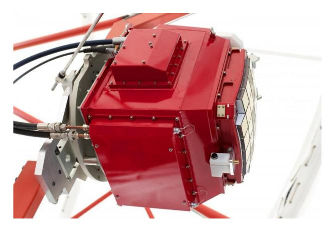
In order to detect the short flashes of light produced by gamma rays as they hit the earth's atmosphere, the telescope's camera has to be about a million times faster than a DSLR camera. To do this, it uses high-speed digitisation and triggering technology capable of recording images at a rate of one billion frames per second and sensitive enough to resolve single photons. Credit: Akira Okumura
