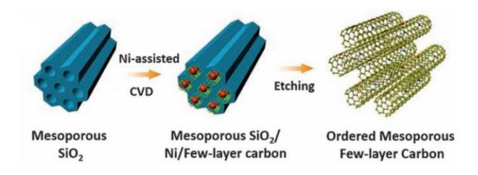
Fabrication schematic of ordered mesoporous fewlayer carbon (OMFLC). Credit: *Science* (2015). DOI: 10.1126/science.aab3798
