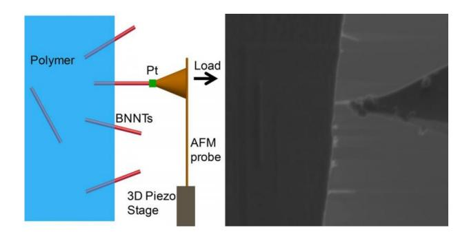
Researchers tested the force required to pluck a boron nitride nanotube (BNNT) from a polymer by welding a cantilever to the nanotube and pulling. The experimental set-up is shown in a schematic on the left and an actual image on the right. Credit: Changhong Ke/State University of New York at Binghamton
