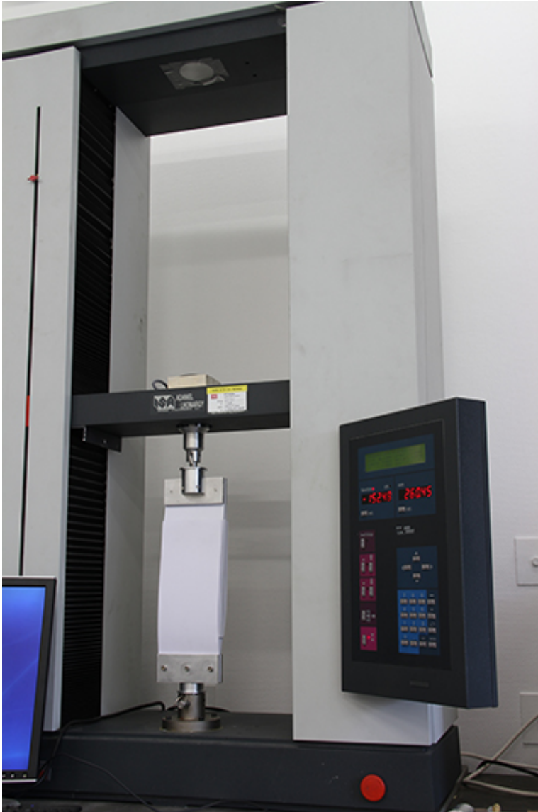
Experimental device used in the laboratory to measure the friction force. Credit: Frédéric Restagno et Christophe Poulard
