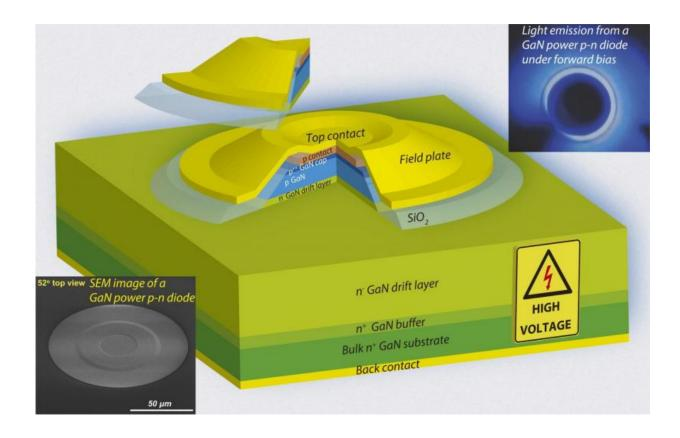
State-of-the-art design of GaN p-n junction diodes that has resulted in near-unity ideality factor, avalanche breakdown capability, and record-breaking power performance. Insets show a GaN p-n diode fabricated on a high-quality bulk GaN substrate and light emission from the junction under forward bias. Credit: Zongyang Hu
