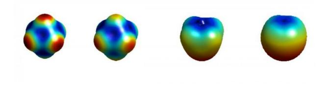
Variations in the energy profile of the crystal under increasing applied electric field, showing a change a phase change in the material. Credit: Credit: Hamidreza Khassaf, University of Connecticut
