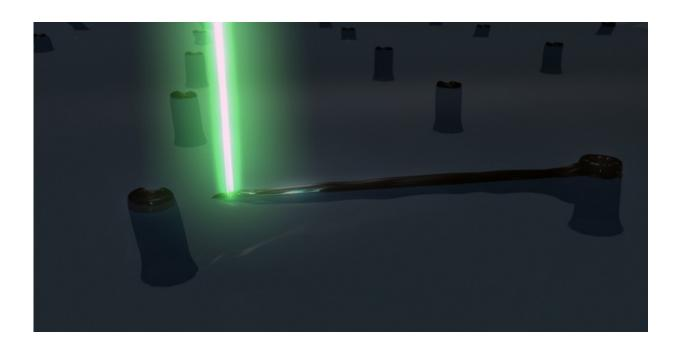
Illustration shows the unique 3D topology of the nanoscale deposit fabricated via bridging "arch" connection between two adjacent nanopillars. Credit: Jeffrey Fisher, Georgia Tech
