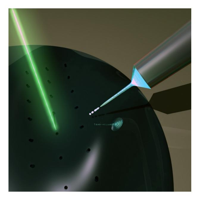
Shown are elements of the NESA-FEBID process involving nanoelectrospray delivery of electrically-energized liquid phase precursor to the substrate where it interacts with an e-beam, resulting in formation of nanoscale deposits. Credit: Jeffrey Fisher, Georgia Tech
