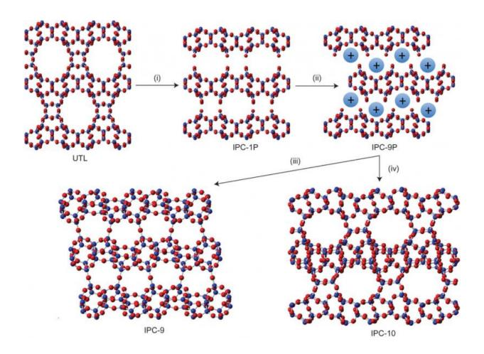
Synthesis of 'unfeasible' zeolites. The ADOR process involves the selective disassembly of a germanosilicate with, in this particular case, the UTL structure to form a layered material (called IPC-1P) (i) followed by the use of the choline cation (shown as a blue circle with a positive charge) as the SDA to shift the layers with respect to each other (IPC-9P) (ii). The layers can then be reassembled in two ways, by calcination to form IPC-9 (iii) and by calcination
