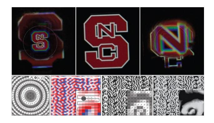
Top Row: Three images of the NC State logo as viewed through a geometric phase hologram, in this case a lens, where each corresponds to one of the three possible wavefronts. Bottom Row: Illustrations, simulation, and microscope picture showing the liquid crystal orientation created by the light patterning techniques reported in the paper, showing a lens profile (left image) and a farfield hologram profile (right three images).
