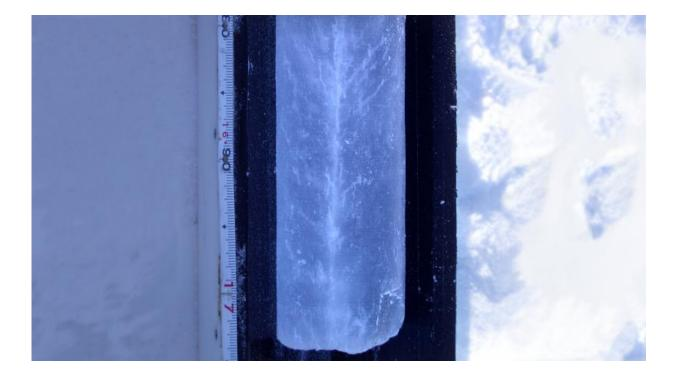
Pathways through sea ice. Ice core taken from Arctic sea ice shows where brine pockets have connected to form channels, with a distinctly visible pathway in the middle. Channels and pathways like these allow sea water or fresh melt water to move, or percolate, through the sea ice. Credit: Ken Golden
