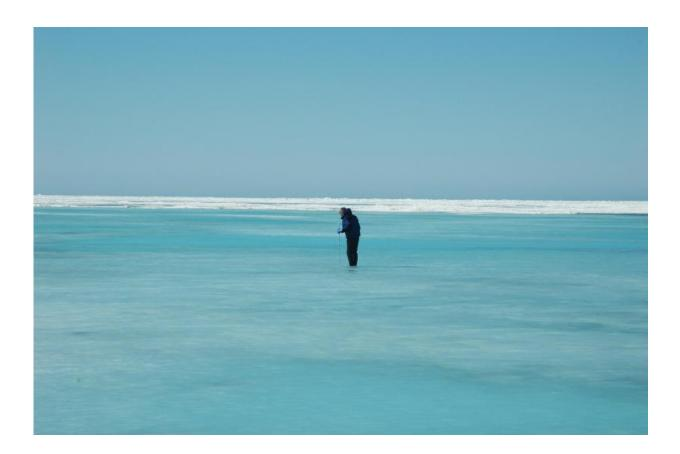
Frogman. A rubber-suited Ken Golden wades into icy Arctic waters to measure the depth of this melt pond. Understanding how environmental conditions like temperature and incoming solar radiation affect percolation, or the movement of water up and down through sea ice, could help scientists better predict how sea ice might respond to changes in its environment. Credit: Don Perovich
