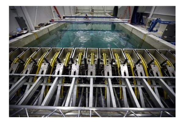
In this Friday, Nov. 20, 2015, photo, paddles that are part of a wave generator line one end of an indoor wave pool and wind tunnel at the University of Maine in Orono, Maine, that is part of the school's expansion of its Advanced Structures and Composites Center. The center's director says with the new equipment, they will be able to simulate a stormy ocean to help innovators find out if their creations can withstand the sea. (AP Photo/Robert F. Bukaty)
