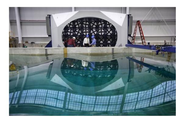
In this Friday, Nov. 20, 2015, photo, waves distort the reflection in an indoor wave pool and wind tunnel at the University of Maine in Orono, Maine. The university's new wind-wave basin is capable of simulating some of the worst conditions at sea at a 1:50 scale. (AP Photo/Robert F. Bukaty)
