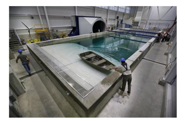
In this Friday, Nov. 20, 2015, photo, a technician steadies a skiff at the "beach" end in an indoor wave pool and wind tunnel at the University of Maine in Orono, Maine. The university's new 90-foot-long wind-wave basin is capable of simulating some of the worst conditions at sea at a 1:50 scale. (AP Photo/Robert F. Bukaty)
