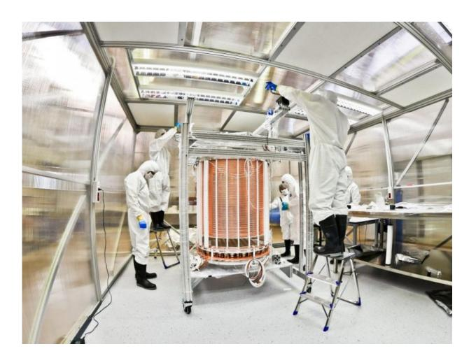
Scientists assemble the XENON1T dark matter detector in the Gran Sasso Underground Laboratory in Italy. UChicago physicist Luca Grandi and his research group played a key role in preparing and assembling the xenon detector. Credit: XENON1T Collaboration
