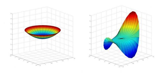
A rotationally symmetric optic is traditionally used in telescopes. The freeform optic on the right takes a different shape and is now being investigated for use in space-based instruments. Credit: NASA
