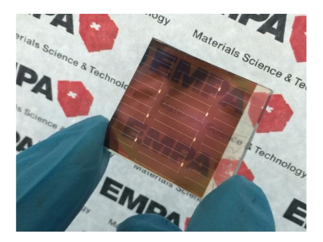
Stacking two solar cells one over the other has advantages: Because the energy is "harvested" in two stages, and overall the sunlight can be converted to electricity more efficiently. Empa researchers have come up with a procedure that makes it possible to produce thin film tandem solar cells in which a thin perovskite layer is used. The processing of
