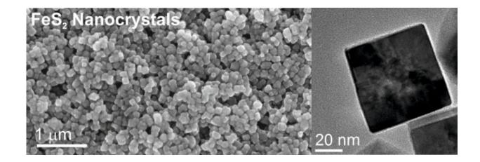
Electronmicroscopical image of Pyrite nanocrystals, which make up the cathode in the fool's gold battery. Credit: Empa
