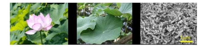
Scientists at Tokyo Institute of Technology have created an ultrathin, light-absorbing 'biometamaterial' using gold sputtered onto a lotus leaf. The natural nano-scale structures on the surface of the leaves created a material with very low reflectivity, which absorbs almost all light on the visible spectrum. Figure: Lotus flower, lotus leaf and scanning-electron microscope image of lotus leaf
