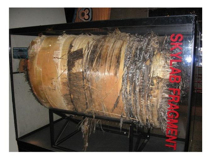
Largest recovered piece of Skylab, on of its six air tanks. Before the crash, it was eight feet long, four feet in diameter and weighted 2,800 pounds empty. Credit: Rycho626/Wikipedia
