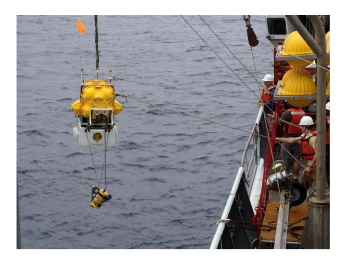
An ocean bottom seismometer being retrieved after spending 10 months on the floor of the Pacific Ocean to map the mantle 100 miles underneath the Juan de Fuca plate. Credit: UC Berkeley
