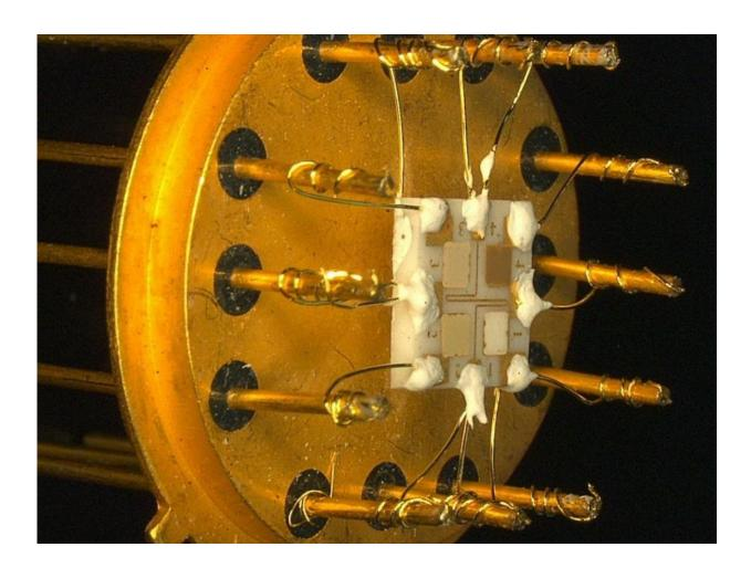
The sensor consists of four areas with different metal oxides. They change their temperature-dependent electric resistance when coming into contact with gases. Credit: KIT/HsKA
