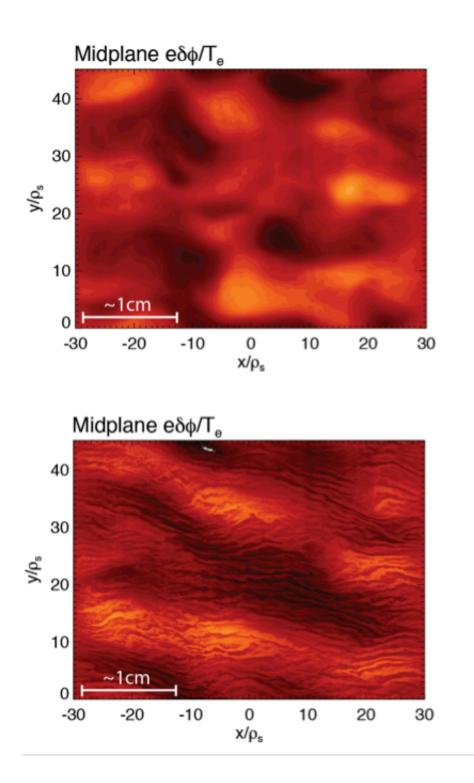
Plasma turbulence in conditions with long wavelength turbulence (top) are compared with those exhibiting long and short wavelength turbulence (bottom). The top condition is representative of the standard model. The bottom model demonstrates the clear impact of capturing long and short wavelength turbulence
