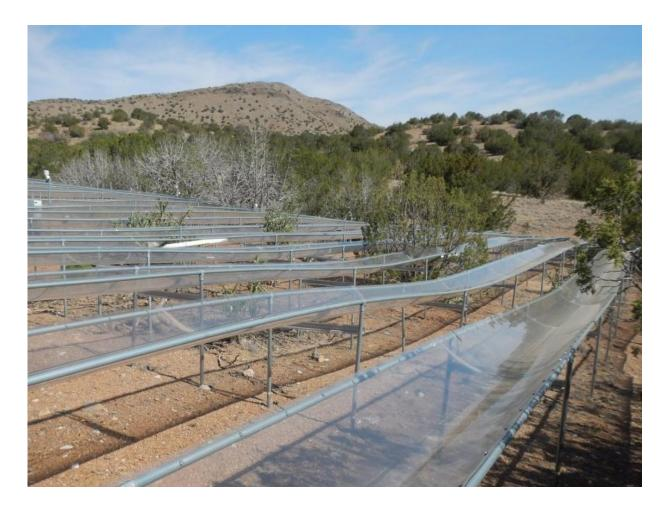
As part of the research, rainfall and temperature were manipulated on 40x40 meter plots assigned to one of four treatments ranging from severe drought to above-average precipitation over a five-year period.
