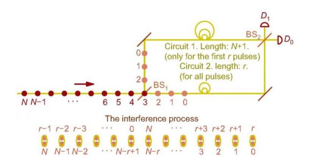
The interference wiring diagram of the newly proposed QPQ protocol, where the database generates a single-photon signal with N optical pulses and shifts the phase of each pulse randomly by 0 or  $\pi$ , then the user extracts the phase differential of two pulses of them by the circuits on the right side and a random number r. Credit: © Science China Press
