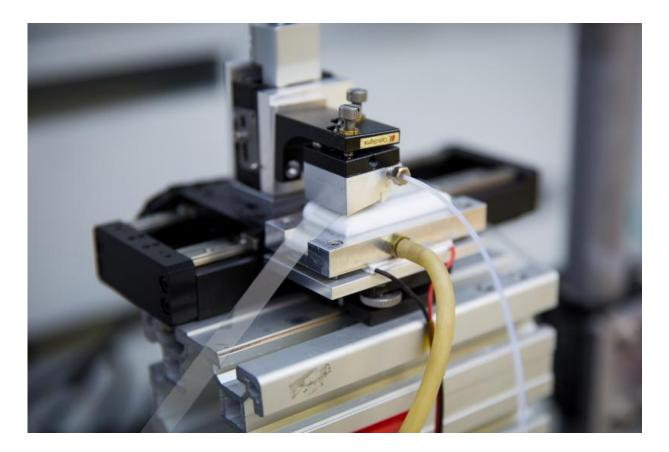
A close-up of the solution shearing apparatus. Transparent conductors made with the technique had record-high electrical conductivity for this material, demonstrating that high performance can be achieved just by controlling the way they are manufactured. Credit: SLAC National Accelerator Laboratory
