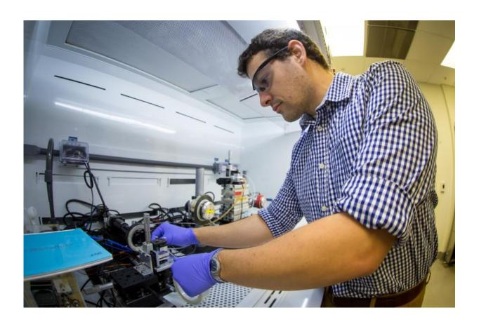
Stanford and SLAC postdoctoral researcher Sean Andrews with an instrument used to spread a thin layer of conductive polymers onto a transparent film with a matchbook-sized silicon blade. The process, called "solution shearing," was used to make patterned electrodes for a solar cell and a sensor, and shows promise for scaling up for use in industry. Credit: SLAC National Accelerator Laboratory
